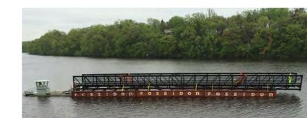
The Poseidon Hopper Barge is made to the same dimensions as the standard barge section. The P2-7' Hopper has male and female connections to allow for the sections to attach to one another or to other Poseidon P2-7' barge sections.
